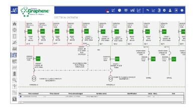
**New!** - "Automatic Line Colouring" automatically define system line colours based on the live status of power cables, energy flow direction, cable's voltage, or breaker status in order to improve the readability of the systems.
