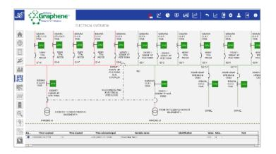
New! - "Automatic Line Colouring" automatically define system line colours based on the live status of power cables, energy flow direction, cable's voltage, or breaker status in order to improve the readability of the systems.
